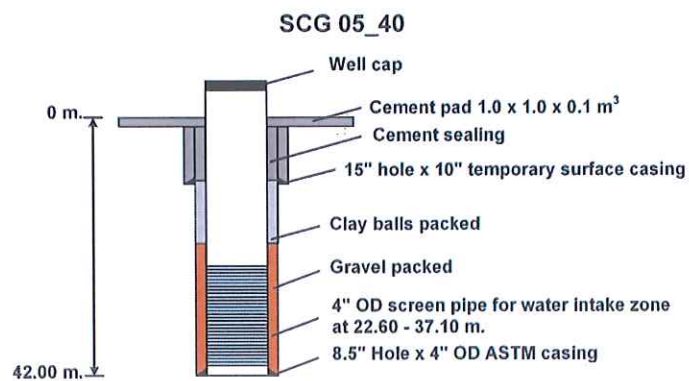
Figure 9 shows the generic well diagram of SCG 05_40.
