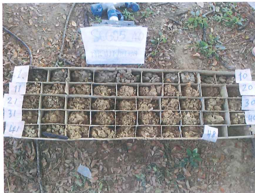
Figure 30 shows drill 8.5" production hole and cutting.
