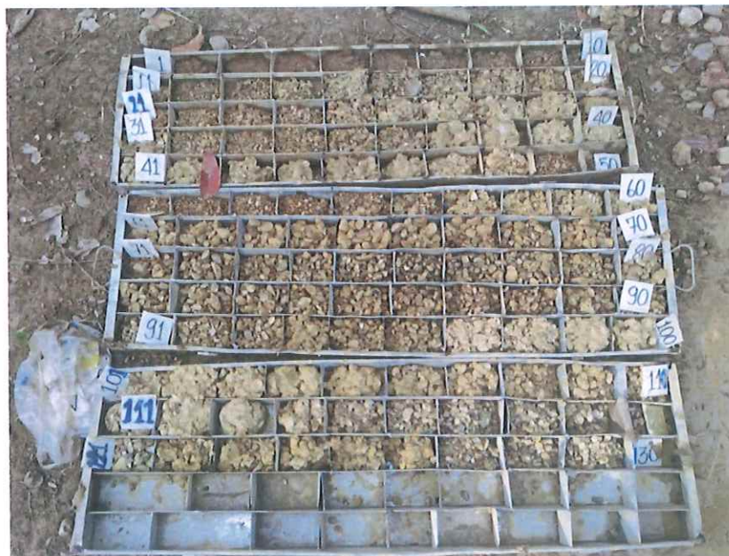
Figure 10 shows drill 8.5" production hole and cutting.
