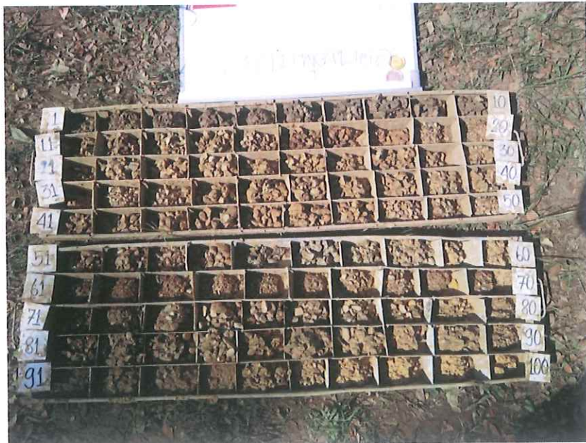
Figure 26 shows drill 8.5" production hole and cutting.
