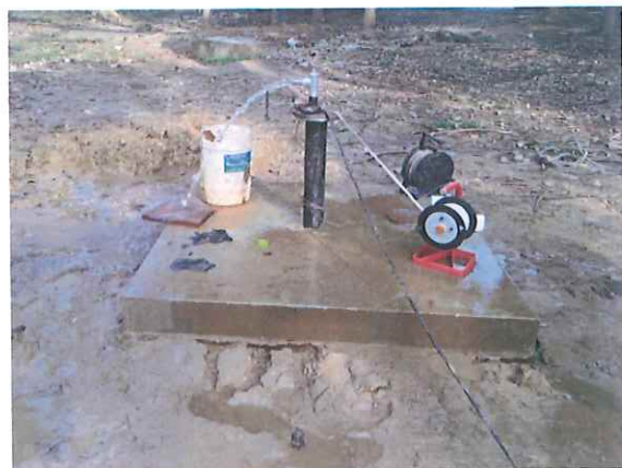
Figure 13 shows completed well and pumping test.
